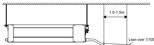
For unit with the drain pump
