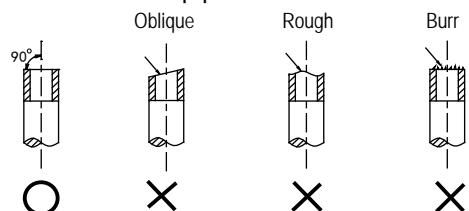
4.1.2 Use a reamer to remove burrs with the cut surface downward so that the chips do not enter the pipe.
