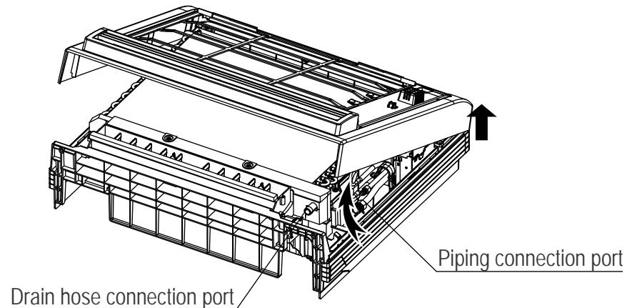
2.3.4 Remove the installation bearer, and take off control box cover. Wiring terminator can be observed.
