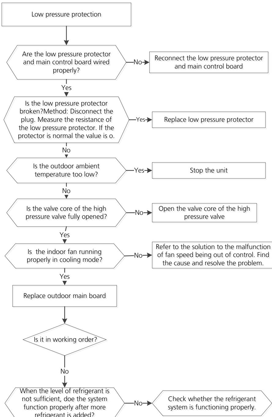
**Note:** For certain models, outdoor PCB could not be removed separately. In this case, the outdoor electric control box should be replaced as a whole.
