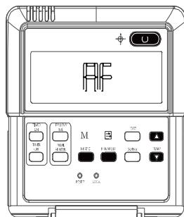
Caution: DO NOT adjust the dampers when automatic airflow adjustment is active.
