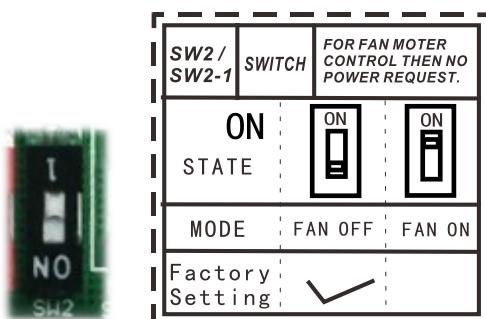
B. Micro-switch SW2/SW2-1 is for selection of indoor FAN ACTION if room temperature reaches the setpoint and the compressor stops.
