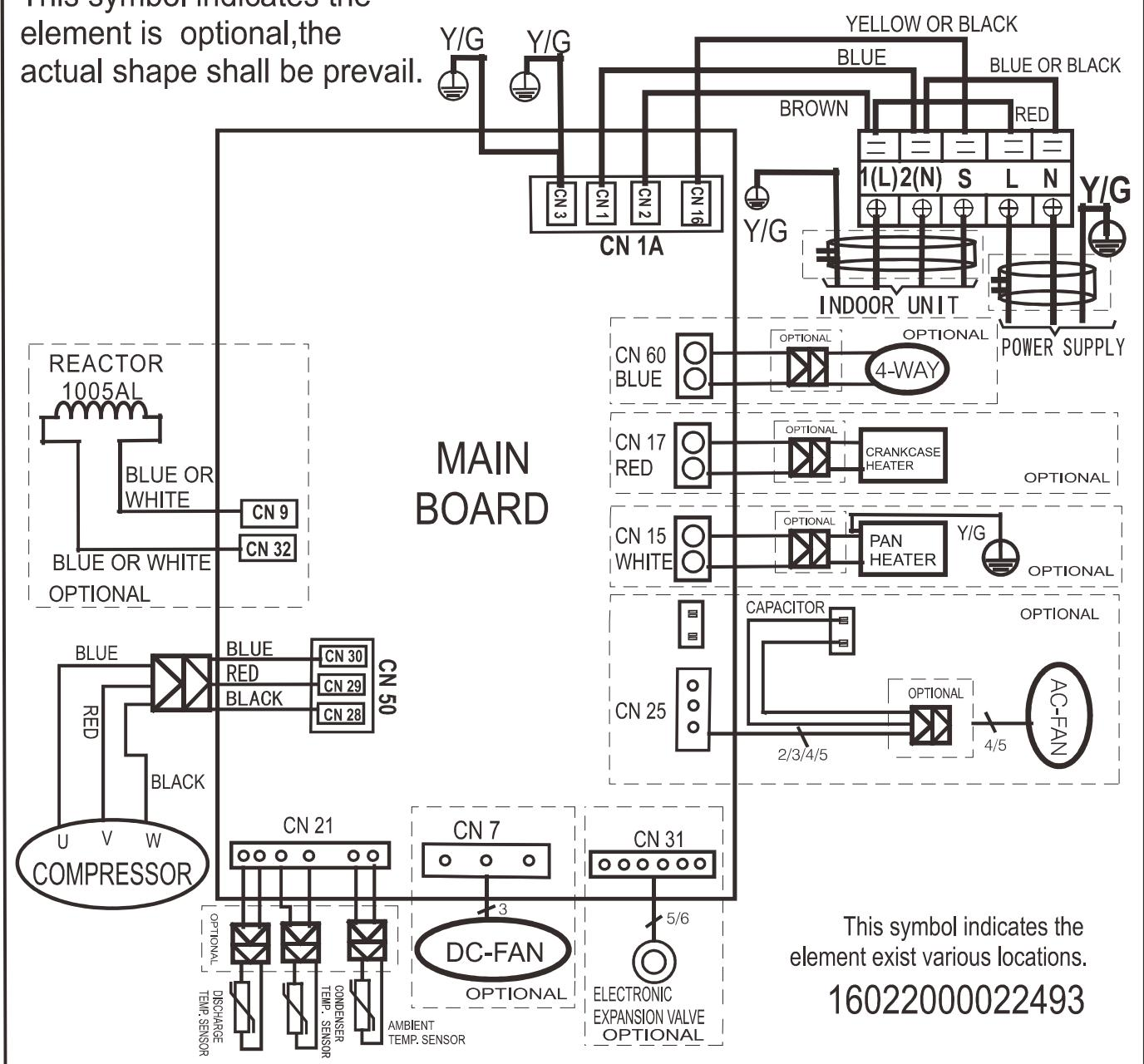
Outdoor unit wiring diagram: 16022000020613
