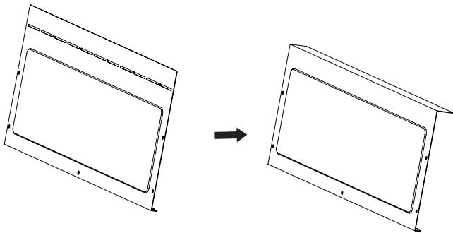
2. Change the mounting positions of ventilation panel and air return flange .
