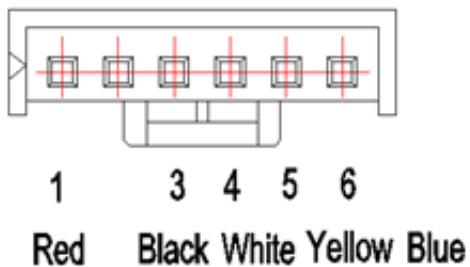
**2. Indoor DC Fan IPM Board (Duct and Ceiling-floor Unit)**
