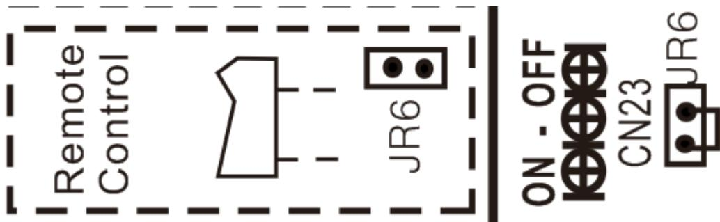
A For remote control (ON-OFF) terminal port CN23 and short connector of JR6
