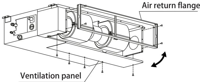
Bend the rear ventilation panel 90 degrees along the dotted line into a descending ventilation panel.(some models)
