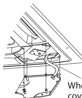
**NOTE:** After installation, the butt plugs of display, swing, water pump and other wire bodies must be placed in the electric control box.
