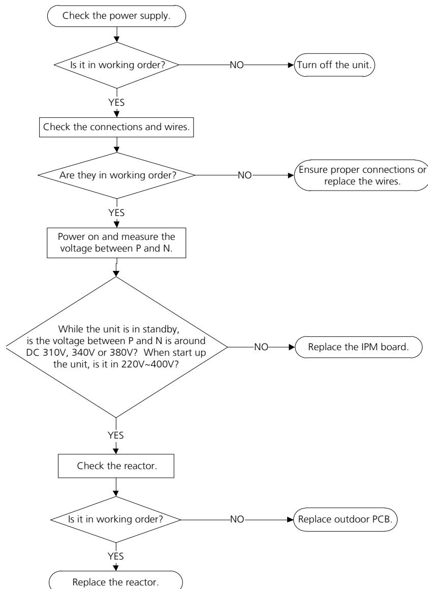
**Note:** For certain models, outdoor PCB could not be removed separately. In this case, the outdoor electric control box should be replaced as a whole.
