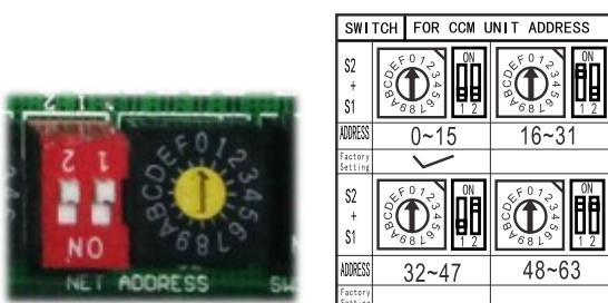
G. Micro-switch S1 and dial-switch S2 are for address setting when you want to control this unit by a central controller.
