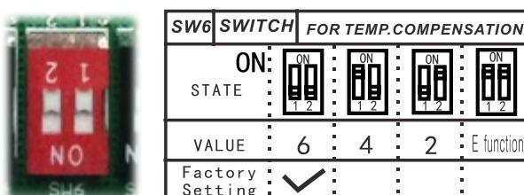
F. Micro-switch SW6 is for selection of temperature compensation in heating mode. This helps to reduce the real temperature difference between ceiling and floor so that the unit could run properly. If the height of installation is lower, smaller value could be chosen.
