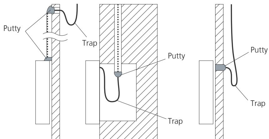
**Note:** DO NOT allow water to enter the remote control. Use the trap and putty to seal the wires.
