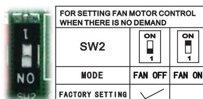
B. Micro-switch SW2 is for selection of indoor FAN ACTION if room temperature reaches the set point and the compressor stops.
