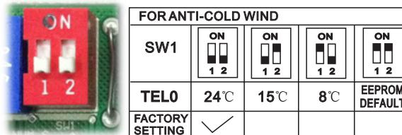
A. Micro-switch SW1 is for selection of indoor fan stop temperature (TELO) when it is in anti-cold wind action in heating mode.
