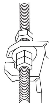
9. Mount the indoor unit onto the hanging screw bolts with a block. Position the indoor unit flat using a level indicator to prevent leaks.
