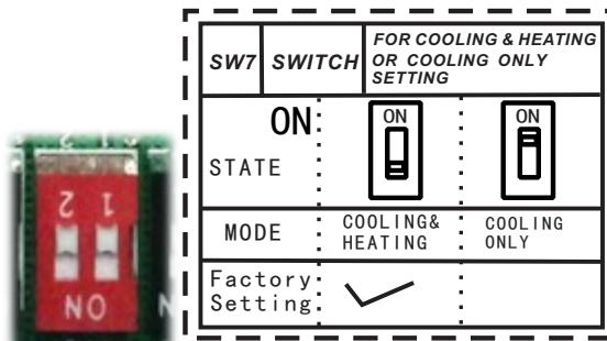
G.Micro-switch SW7 is for setting cooling &heating or cooling only.
