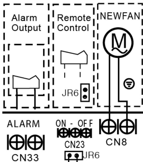
A For remote control (ON-OFF) terminal port CN23 and short connector of JR6
