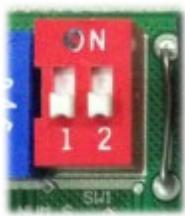
A. Micro-switch SW1 is for selection of indoor fan stop temperature (TEL0) when it is in anti-cold wind action in heating mode.
