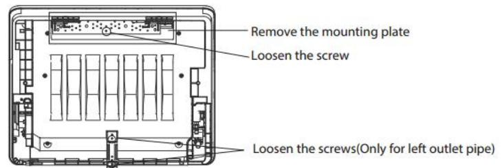
NOTE: If the pipe comes out on the left, it is necessary to loosen the screws on the bottom mounting. If the pipe comes out in other directions, it is not necessary.
