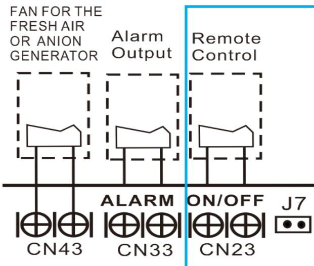
C. For remote control (ON-OFF) terminal port CN23 and short connector of J7
