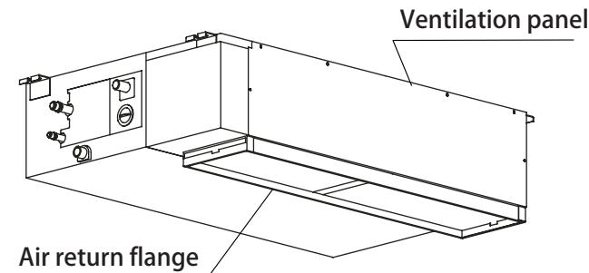
3. When installing the filter mesh, fit it into the flange as illustrated in the following figure.
