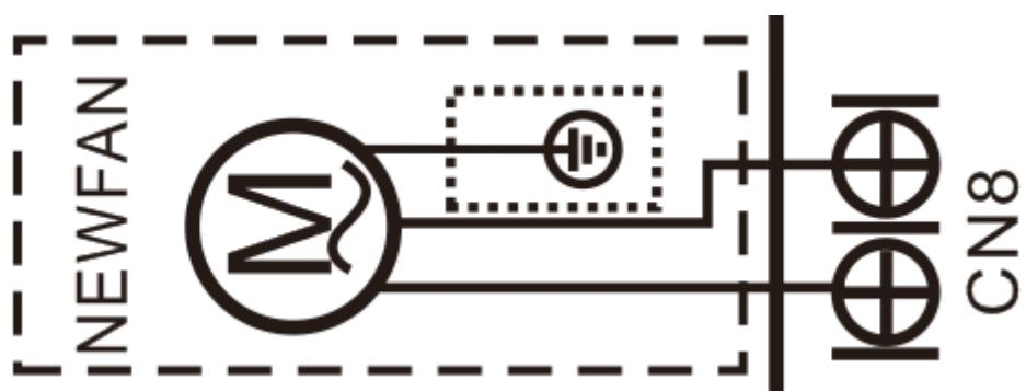
C. For new fresh motor terminal port CN8
