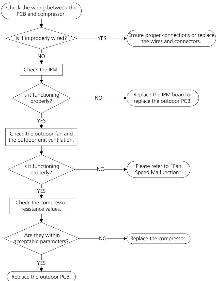
**Note:** For certain models, outdoor PCB could not be removed separately. In this case, the outdoor electric control box should be replaced as a whole.
