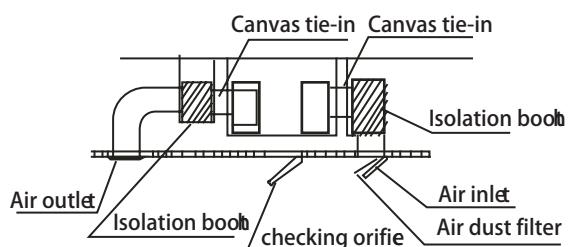
5. For DC motor models, you can change the fan motor static pressure according to external duct static pressure.
