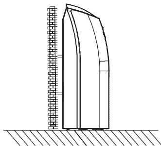
8. Mount the indoor unit onto the hanging screw bolts with a block.
