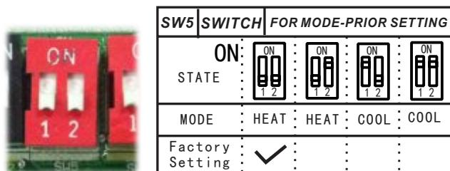
E. Micro-switch SW5 is for setting mode priority of multi connection.
