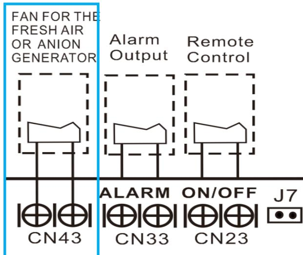
A. For new fresh motor terminal port (also for Anion generator) CN43:
