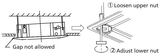
If the unit is not hung correctly and a gap exists, the unit's height must be adjusted to ensure proper function. The unit's height can be adjusted by loosening the upper nut, and adjusting the lower nut.
