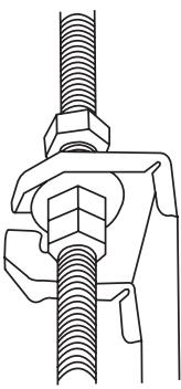
D. Refrigerant pipe connection (D.gas side)
