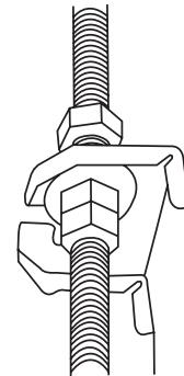
Adjust the position to ensure the gaps between the indoor unit and the four sides of false ceiling are even. The bottom of the unit should be 10 - 25mm (0.4-0.98") higher than ceiling board. Generally, L should be half the length of the suspension bolt or long enough to prevent the nuts from coming off.
