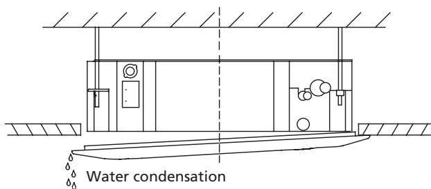
Failure to tighten screws can cause water leakage.
