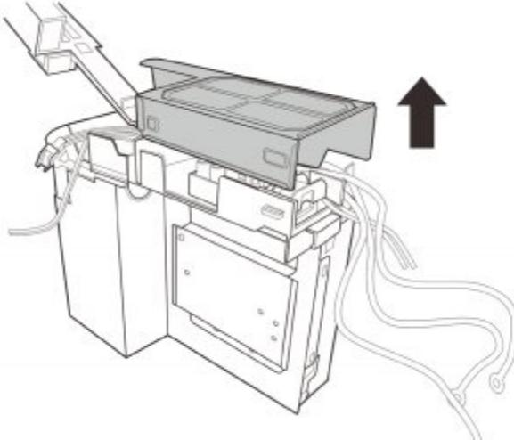
A line drawing of a rectangular component with internal compartments. A grey rectangular board is positioned above one of the compartments. A large black arrow points upwards, indicating the direction of removal for the fixing board. |
