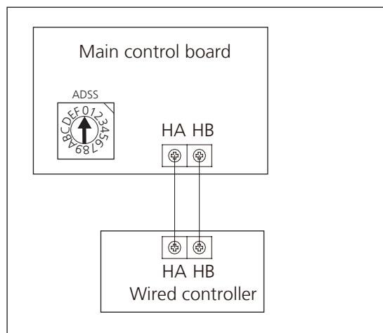
For Duct, Ceiling& floor: The wired controller connects to terminal board, terminal board connects to main control board.
