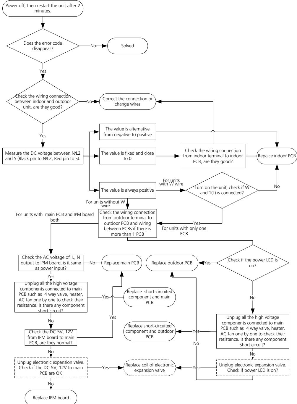
**Note:** For certain models, outdoor PCB could not be removed separately. In this case, the outdoor electric
